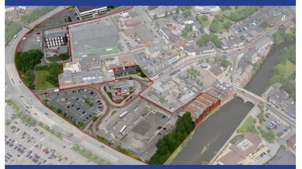
Low carbon infrastructure for Bury, Prestwich and Radcliffe: Identifying low carbon infrastructure opportunities to supply new and existing buildings in and around district centres in Bury. Technologies include wind power, gas fired CHP, biomass heating, wastewater treatment heat recovery, minewater geothermal heating, hydroelectric and micro-generation.
