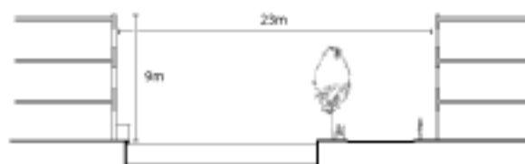
Section 1: 1:500 Typical Section through proposed IPL Masterplan showing ratio of open space to building height. This would allow lots of natural daylight into the canal and not produce a canyon effect, for comparison with section below.
