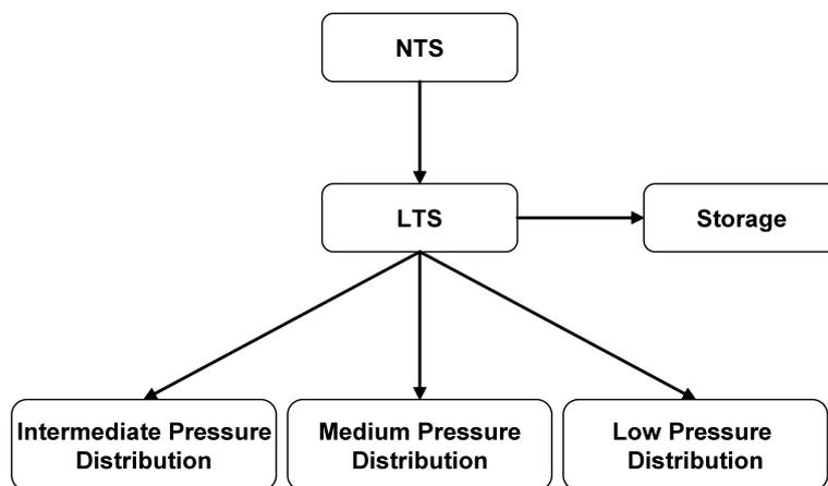
The High Pressure (LTS) system does not enter city centre areas. Most developments will receive gas from the low pressure mains, if this causes constraints it may be possible to connect to medium pressure mains nearby dependent on location, cost and complexity (e.g. railways or other obstacles). Although the mains pressure can cause constraints for developments and CHP, the system is more flexible than the electricity network because it is possible to store gas to cope with the demand peaks.
